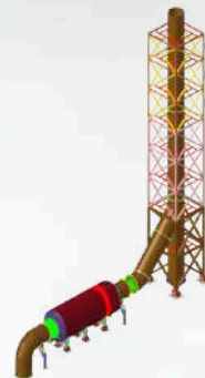
Exhaust Duct Lattice Structure
