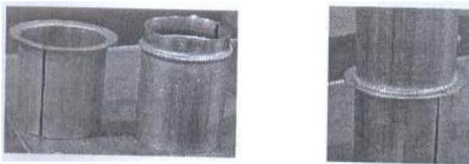
Figure.2 Tube with a flange (left) and a tube with a fold right for welding shown with a Welded tube.
