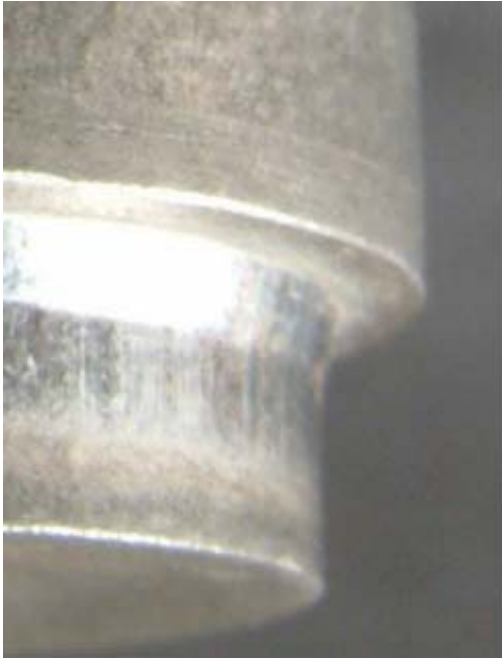
Figure 4a Underfill in the forged component
